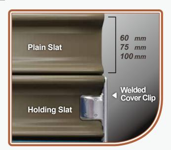
Traditional Roller Shutter are arranged with two different types of slats. One type is a "plain slat" (plain from end to end). The other is a plain slat with a metal, welded "cover clip" (explained below). These 2 slats alternate on the door. The slat heights can be either 60, 75 or 100 mm. This is the only slat arrangement for Traditional Roller Shutters.
