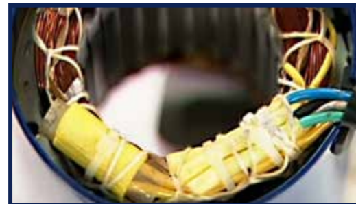
Motor temperature Sensor - Overheat Auto-Stop
