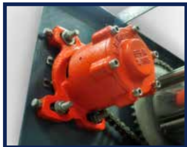
Emergency brake mechanism in case of chain failure (optional)
